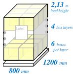
Articles in a pile: 50 Piles in a box: 25 Articles in a box: 1250 Box inner size: 392x392x480 Box load gross: 11,08 kg Boxes per pallet: 24 Articles per pallet: 30000 Pallet height: 2,13 m
